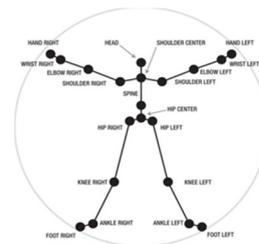
Figure 6 The skeleton joints of the Kinect
