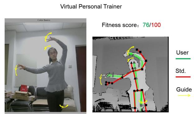
**Figure 3** The proposed Virtual Personal Trainer. The left is the user video captured by the camera of the Kinect. The right is the real time skeleton of the user (shown in green lines) and the matched standard skeleton (shown in red lines). The fitness score is shown above the skeleton in real time. The action correction guide in 3D space is shown in both the user video and the skeleton video.
