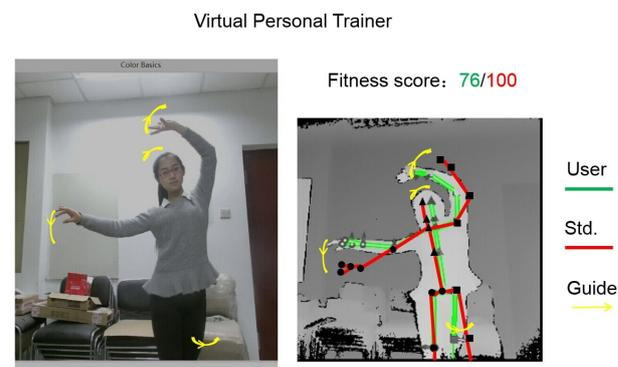
**Figure 3** The proposed Virtual Personal Trainer. The left is the user video captured by the camera of the Kinect. The right is the real time skeleton of the user (shown in green lines) and the matched standard skeleton (shown in red lines). The fitness score is shown above the skeleton in real time. The action correction guide in 3D space is shown in both the user video and the skeleton video.
